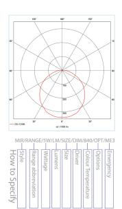
To Specify: CASPER LED, 18.7W, Ø351mm, 1951lm, 4000k, LED surface mounted finished black supplied with hood attachment and complete with standard control gear. Part code: MI/CASP/18.7W/1951lm/840/BK/HD
